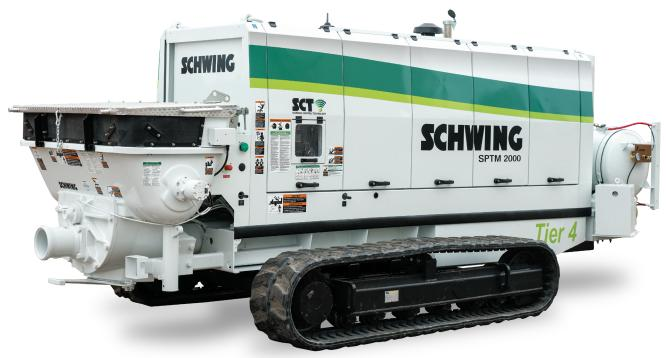
Foundation contractors and rough terrain applications will benefit from SPTM track-mounted concrete pumps. For contractors drilling multiple cast piles, the SPTM is self-propelled to eliminate a tow vehicle with operator. The two-speed hydraulically powered track system navigates 42% grades at up to 4.6 mph allowing it to follow drill rigs to perform concrete pumping of cast-in-place pilings.
