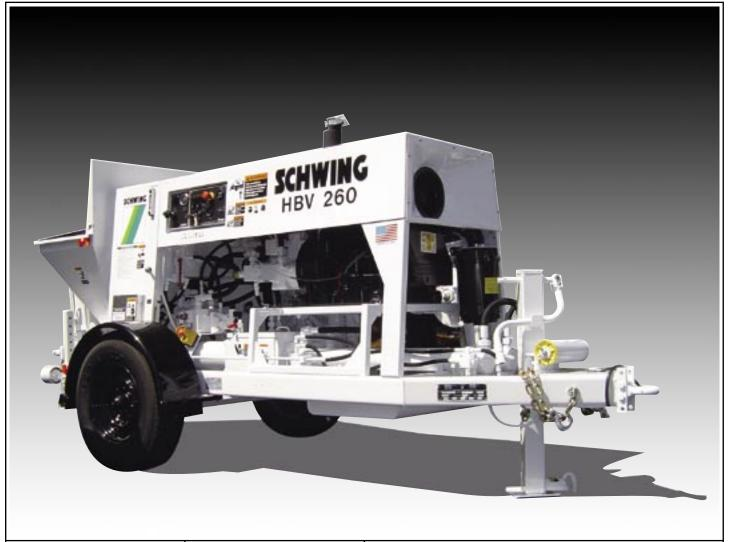
Schwing brings hydraulic actuation to ball valve simplicity at an economical price with the HBV-260. Exceptional distances can be reached with the 1100-psi pumping pressure. Most important, proven Schwing hydraulics guarantee longterm, trouble-free operation with minimal maintenance. Ball valve sequencing of the hopper and twin cylinders is the simple, easy to maintain method that appeals to most grout pumpers. The out-
