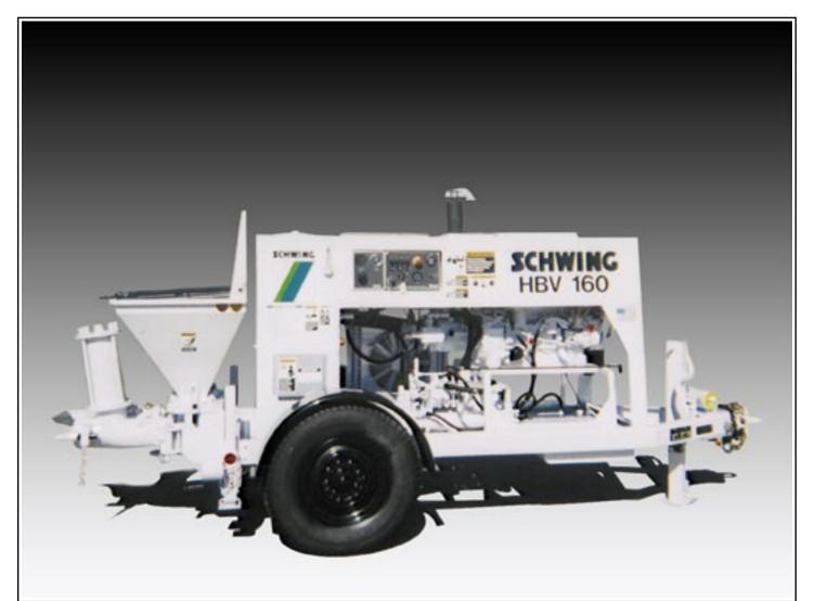
Schwing brings hydraulic actuation to ball valve simplicity at an economical price with the HBV-160. Exceptional distances can be reached with the 1100-psi pumping pressure. Most important, proven Schwing hydraulics guarantee long-term, trouble-free operation with minimal maintenance. Ball valve sequencing of the manifold and twin cylinders is the simple, easy to maintain method that appeals to most grout pumpers. The outlet manifold is fitted with
