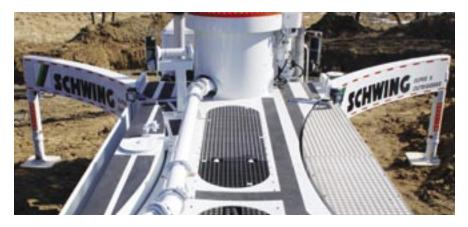
Super X outriggers are a Schwing exclusive providing maximum stability with the smallest footprint. These telescopic, single-stage outriggers set-up fast and don't extend in front of the cab for maximum horizontal boom reach.
