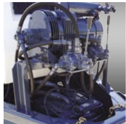
Optional, hydraulically powered air compressor is mounted on front of pump for easy access and provides 30 CFM @ 140 psi for system cleanout and other jobsite duties.
