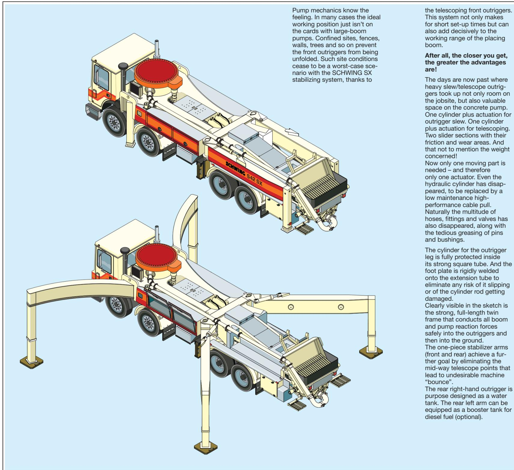
Pump mechanics know the feeling. In many cases the ideal working position just isn't on the cards with large-boom pumps. Confined sites, fences, walls, trees and so on prevent the front outriggers from being unfolded. Such site conditions cease to be a worst-case scenario with the SCHWING SX stabilizing system, thanks to
